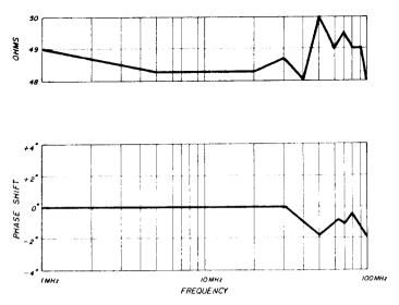
fig. 5. Impedance characteristics of the broadband reflectometer, as measured with a Hewlett-Packard vector voltmeter while terminated with a 50-ohm load.
